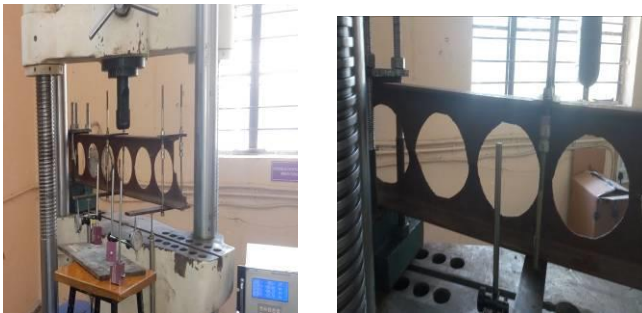
Fig. Lateral torsional buckling on NPI-125 (Circular)
