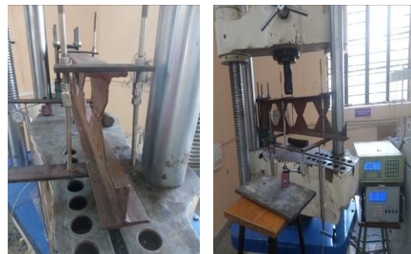
Fig. Lateral torsional buckling on NPI-125 (Hexagonal)
