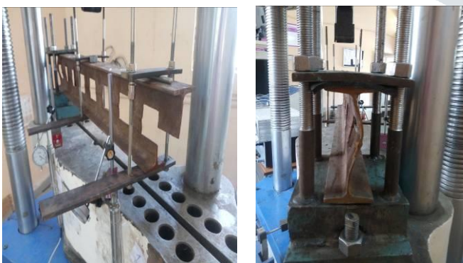
Fig. Lateral torsional buckling on NPI-125 (Square)
