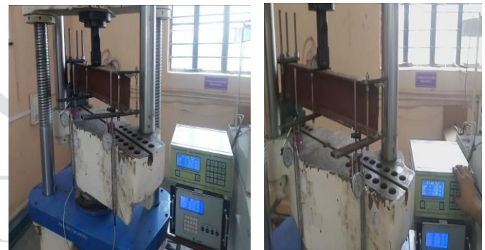
Fig. Lateral torsional buckling on NPI-125 (Plane)
