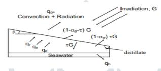
Heat flux from the water to the cover by radiation Qr can be estimated using the relation planes. The radiation involved is considered as diffuse radiation in long wavelengths, so that specular reflection between the transparent cover and water surface is negligible. As a result, the shape factor can be closely approximated by the emissivity of the water surface, usually taken as 0.9 for the conditions inside the still.
