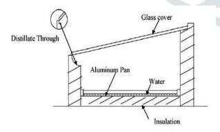
This is the basic model. Over decades several other designs mostly based on variations in the geometric configurations have been developed to improve the efficiency of passive basin type solar stills (Hamed et al., 1993). Shankar and Kumar (2012) summarize the solar distillation systems n the broad category of solar stills, it is classified into passive and active distillation systems (Tiwari et al., 2003). In active systems, an external source (such as a flat plate or concentrator collector)
