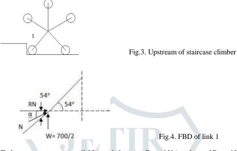
Note :- To have net +ve torque available, angle between  $R_N$  and N (resultant of  $R_N$  and W)
