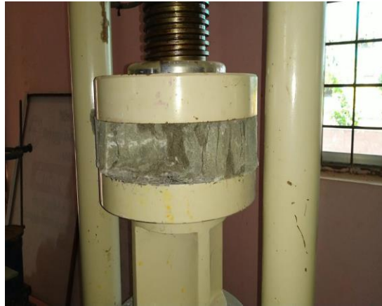
6. Fig. compressive strength test
