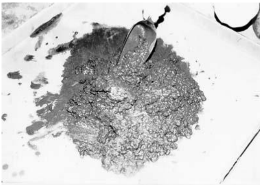
3. Fig. mixing sand, stone, cement and water
