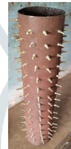
Figure 11 Spirally bolted threshing drum
