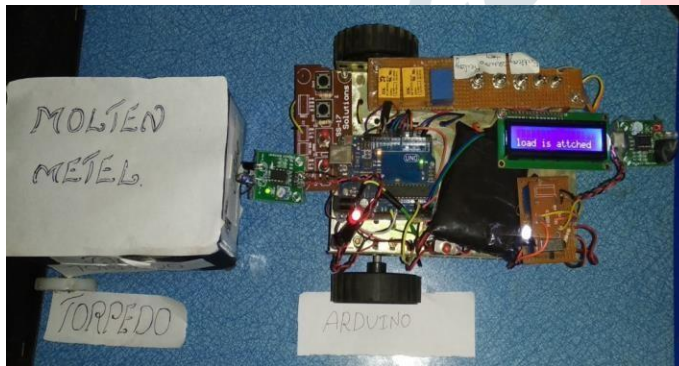
Picture 2: Display showing that load is attached and two LEDs are in on condition. LEDs are indicating that two engines are in on position.
