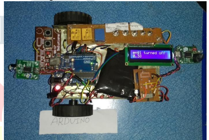
Picture 4: More than five minutes if load was not connected, arduino checks the condition of alternator battery voltage idle relay if this condition is satisfied one engine gets shutdown.
