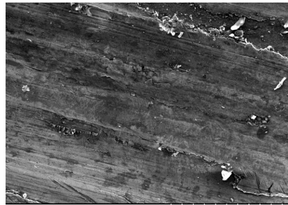
Fig.6: SEM micro graph of 0.2% Mn as received specimen, Speed-2.5 m/s, Nr. Pressure 0.49962 MPa
