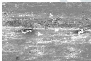
Fig.10.SEM micro graph of Sp-4, Speed-2.45m/s, applied load 20 N.
