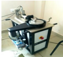
Fig.4. Ducom pin on Disc sliding wear test apparatus.
