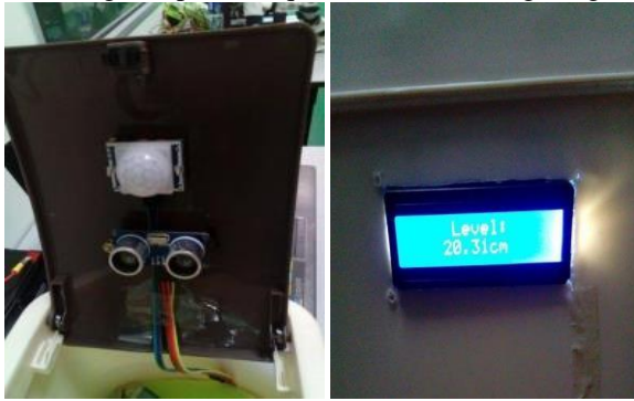
Fig. 4: Sensors attached at the waste bin lid.
