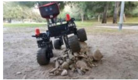
NASA's *Open Source Rover* powered by a Raspberry Pi 3.
