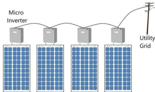
Fig. 5. Micro Inverter Topology
