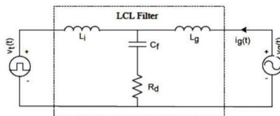
Fig. 6. LCL Filter and Components
