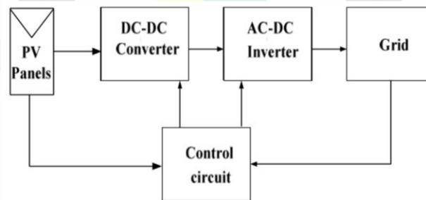
Fig. 1. Block diagram of a grid connected PV system
