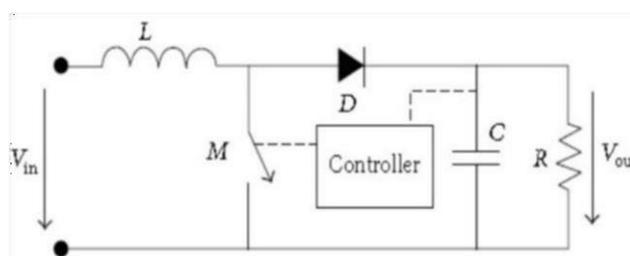
Fig. 2. Circuit topology of DC boost converter
