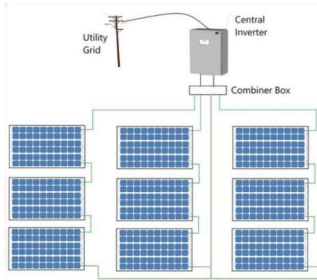
Fig. 3. Grid Connected Centralised Inverter System
