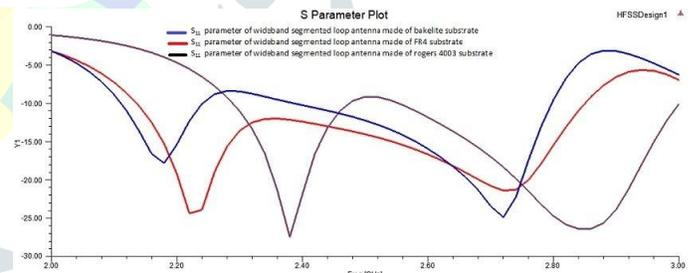
Fig. 3. S-parameter plot of wideband segmented loop antennas made of Bakelite, FR4, Rogers 4003.
