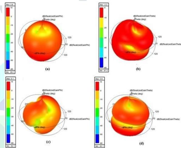
Fig. 8. Simulated 3D radiation patterns of wideband segmented loop antenna made of FR4 substrate. (a) Horizontally polarized pattern at 2.2 GHz. (b) Vertically polarized pattern at 2.2 GHz. (c) Horizontally polarized pattern at 2.8 GHz. (d) Vertically polarized pattern at 2.8 GHz.
