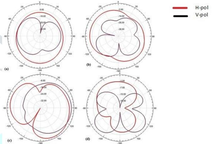
Fig. 11. Simulated 2D radiation patterns of wideband segmented loop antenna made of FR4 substrate. (a) XY plane radiation patterns at 2.2 GHz. (b) XZ plane radiation patterns at 2.2 GHz. (c) XY plane radiation patterns at 2.8 GHz. (d) XZ plane radiation patterns at 2.8 GHz.
