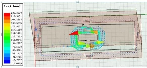
Fig. 4. The current distribution of segmented loop at 2.2 GHz.
