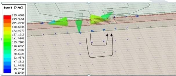
Fig. 6. The current distribution of ground plane at 2.2 GHz.
