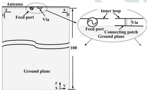
Fig. 2. Antenna geometry side view.
