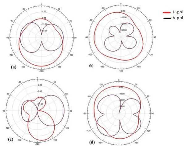
Fig. 13. Simulated 2D radiation patterns of wideband segmented loop antenna made of Rogers 4003 substrates. (a) XY plane radiation patterns at 2.2 GHz. (b) XZ plane radiation patterns at 2.2 GHz. (c) XY plane radiation patterns at 2.8 GHz. (d) XZ plane radiation patterns at 2.8 GHz.
