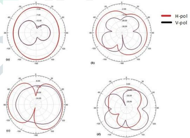
Fig. 12. Simulated 2D radiation patterns of wideband segmented loop antenna made of Bakelite substrate. (a) XY plane radiation patterns at 2.2 GHz. (b) XZ plane radiation patterns at 2.2 GHz. (c) XY plane radiation patterns at 2.8 GHz. (d) XZ plane radiation patterns at 2.8 GHz.
