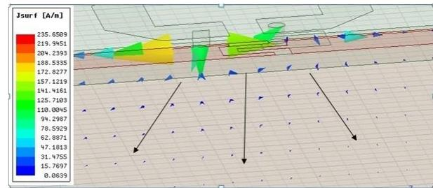
Fig. 7. The current distribution of ground plane at 2.8 GHz.
