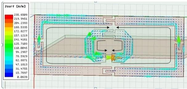
Fig. 5. The current distribution of segmented loop at 2.8 GHz.
