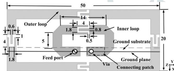
Fig. 1. Antenna geometry top view.
