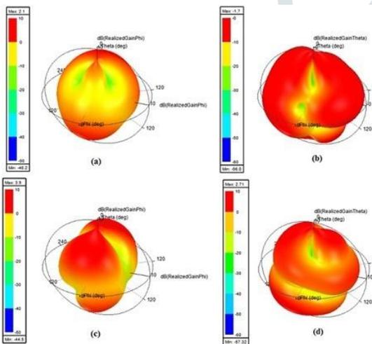
Fig. 10. Simulated 3D radiation patterns of wideband segmented loop antenna made of Rogers 4003 substrates. (a) Horizontally polarized pattern at 2.2 GHz. (b) Vertically polarized pattern at 2.2 GHz. (c) Horizontally polarized pattern at 2.8 GHz. (d) Vertically polarized pattern at 2.8 GHz.
