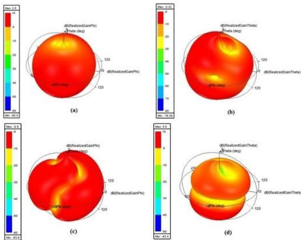
Fig. 9. Simulated 3D radiation patterns of wideband segmented loop antenna made of Bakelite substrate. (a) Horizontally polarized pattern at 2.2 GHz. (b) Vertically polarized pattern at 2.2 GHz. (c) Horizontally polarized pattern at 2.8 GHz. (d) Vertically polarized pattern at 2.8 GHz.
