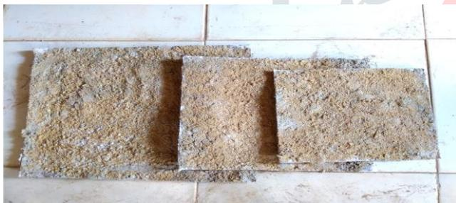
Figure 1.Geotextile with cement interface
