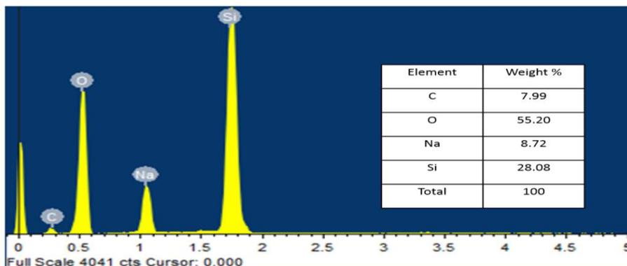
Fig.6. EDX of nanosilica particles.
