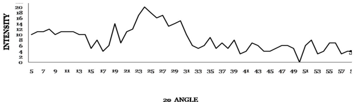
Fig.4. X –Ray Diffractogram of nanosilica.
