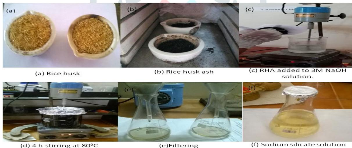
Fig.1. Preparation of sodium silicate solution from rice husk
