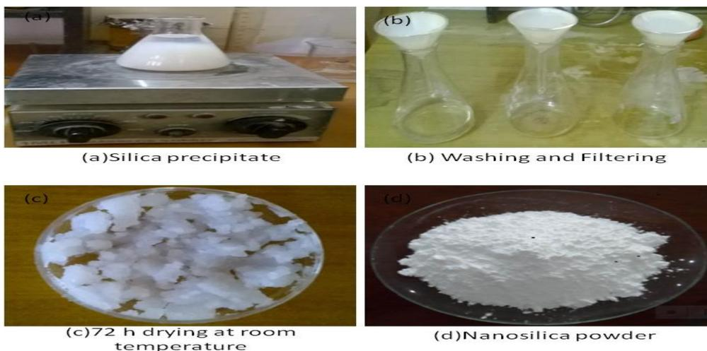
Fig.2.Synthesis of nanosilica by precipitation method
