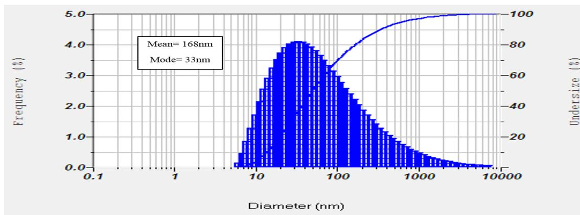
Fig.7. DLS analysis of nanosilica particles
