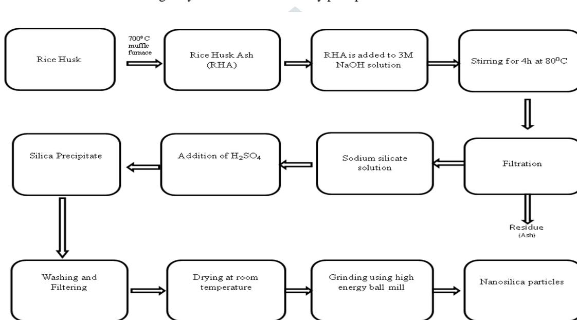
Fig.3. Flowchart for preparation of Nanosilica by precipitation method
