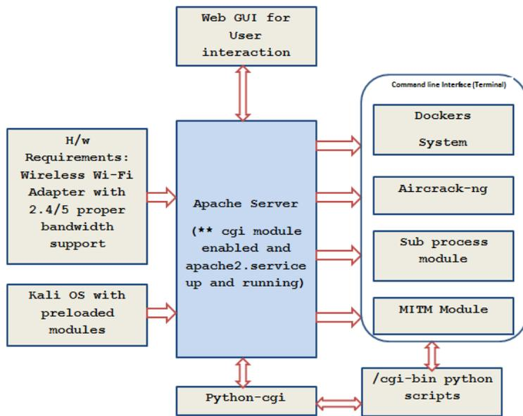
Figure 2. Architecture Diagram of DEADSEC
