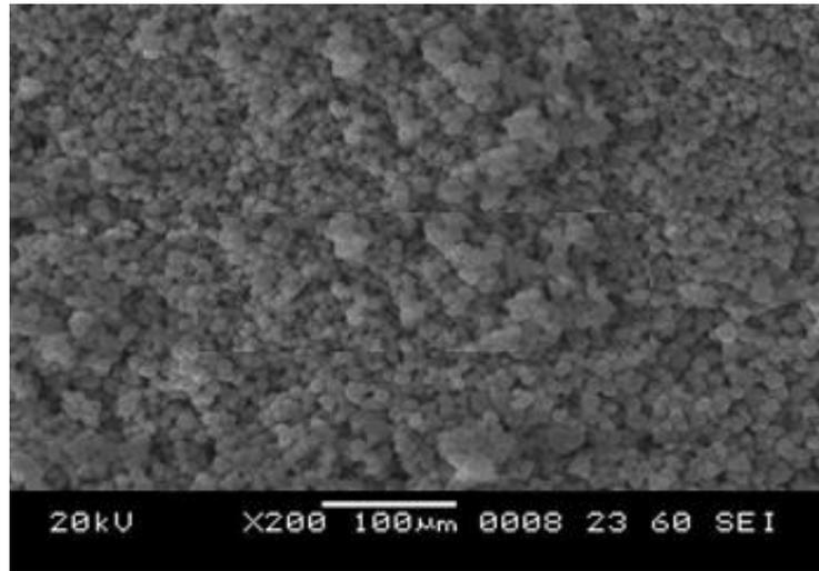
Figure2. SEM micrographs of BaTiO<sub>3</sub> thin film
