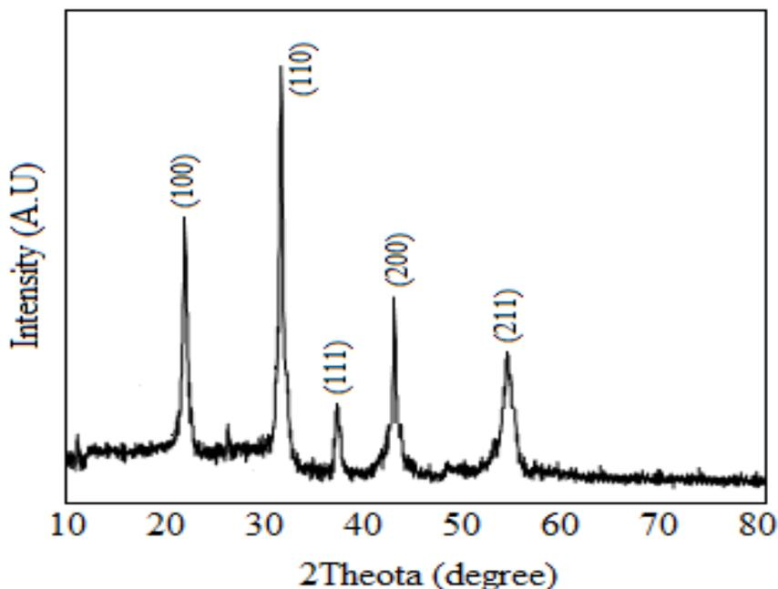
Figure1. XRD pattern of BaTiO<sub>3</sub> thin filmTable1: Comparison of observed and standard XRD data of BaTiO<sub>3</sub> thin films (JCPDS card 31-0174).
