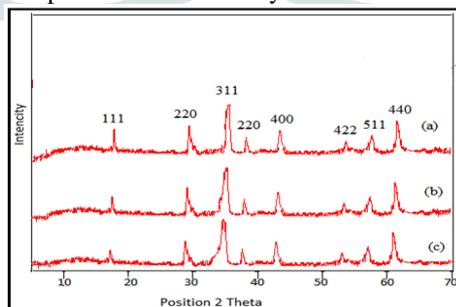
**Figure 1 X-ray diffraction patterns for (a) 1 wt %, (b) 2 wt% and (c) 3 wt% Ag doped CuFe<sub>2</sub>O<sub>4</sub> NPs calcined at 350°C.**
