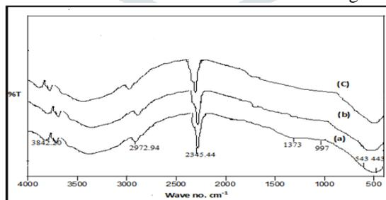
**Figure 2 FTIR Spectra for (a) 1 wt% (b) 2 wt% and (c) 3 wt% Ag doped CuFe<sub>2</sub>O<sub>4</sub> NPs calcinate at 350°C.**
