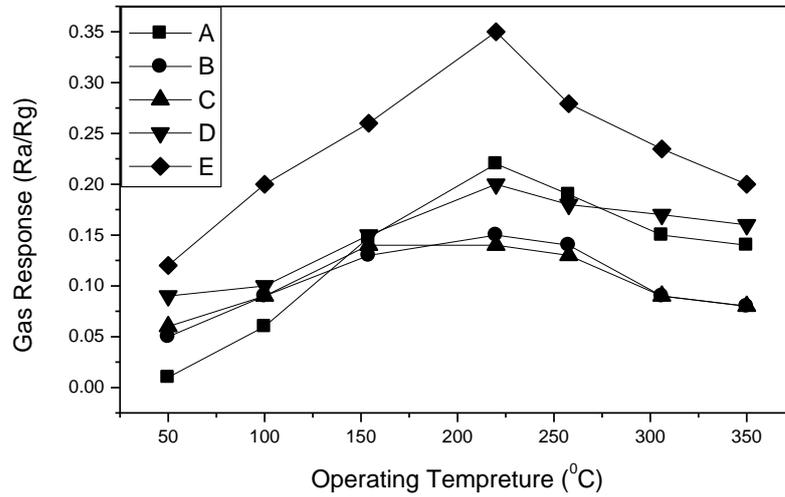
**Figure 3:** Gas Response of  $\text{CoFe}_2\text{O}_4$  doped with different amount of Zn (A)  $x=0$ , (B)  $x=0.2$ , (C)  $x=0.4$ , (D)  $x=0.6$  and (E)  $0.8$
