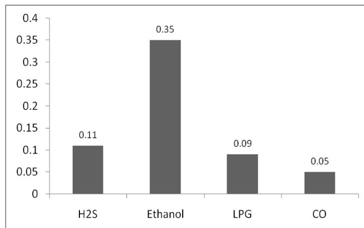
**Figure 6: Response to different reducing gases of 0.8 wt% Zn-doped  $\text{CoFe}_2\text{O}_4$  as a function of operating temperature.**
