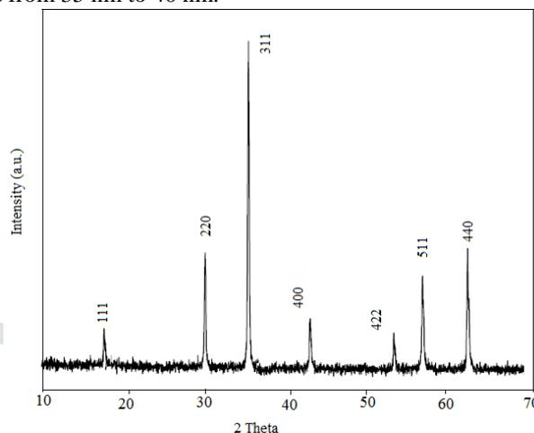
**Figure 1. X-ray Diffraction pattern of  $\text{Co}_{0.2}\text{Zn}_{0.8}\text{Fe}_2\text{O}_4$  nanoparticles calcined at 700 °C**
