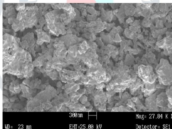
**Figure 2. SEM image of  $\text{Co}_{0.2}\text{Zn}_{0.8}\text{Fe}_2\text{O}_4$  nanoparticles calcined at 700 °C**
