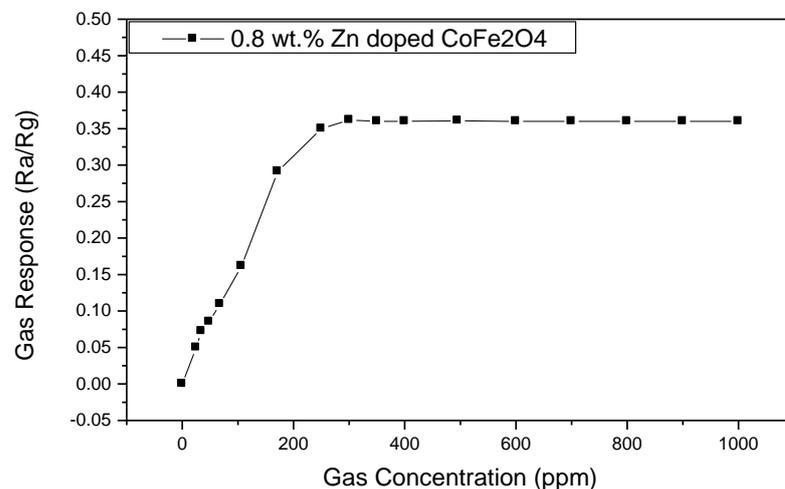
**Figure 5:** Response of  $0.8 \text{ wt}\%$  Zn-doped  $\text{CoFe}_2\text{O}_4$  to Ethanol gas of different concentration at an operating temperature  $220^\circ\text{C}$ .
