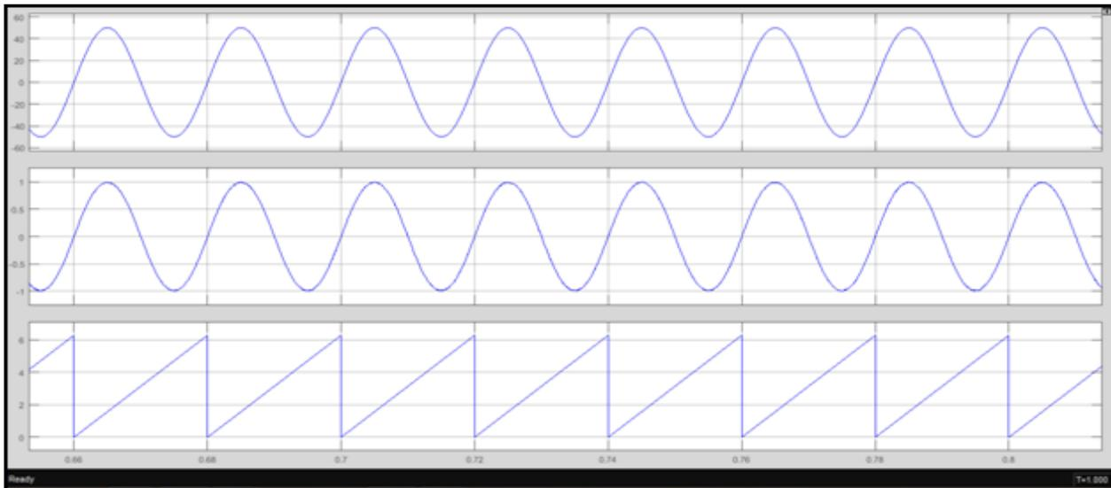
Figure2 Shows the Grid voltage and current along with PLL behavior.
