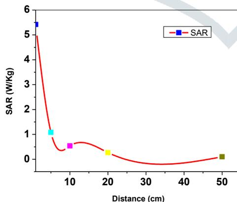
**Figure1: Variation of Specific Absorption rate with distance from mobile phone.**
