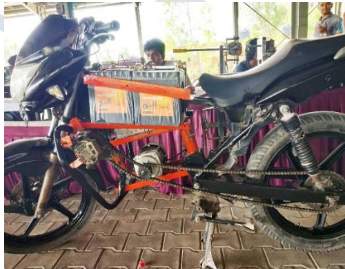
Figure(d): Final assembly of Regenerative E-bike
