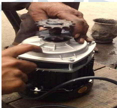
Figure(b): BLDC hub motor with two sprockets
