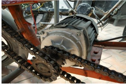
Figure(c): Double Chain Mechanism
