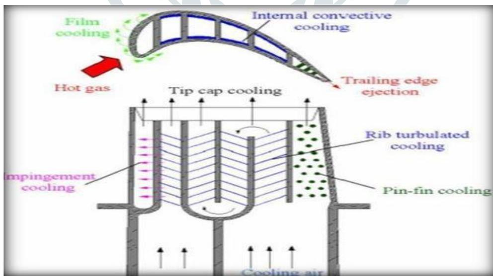
**Fig.2** Internal convective cooling [5]
