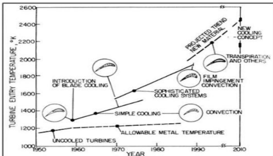
Fig 5: Cooling technology for gas turbine blades [22]
