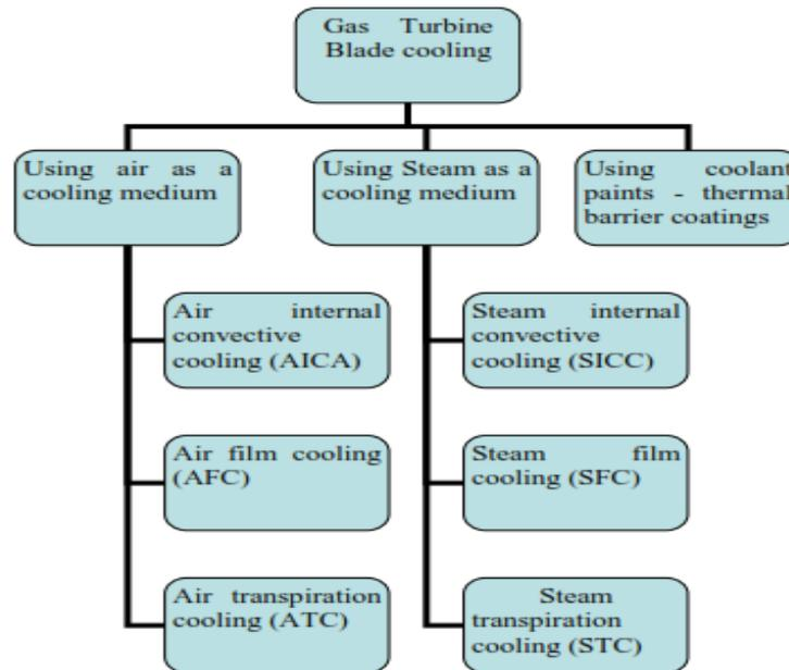
**Fig.1** Classification of the blade cooling
