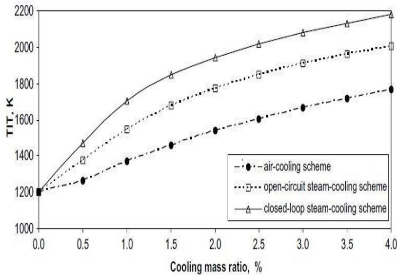
Fig 7. Variation of TIT with cooling mass ratio [7]
