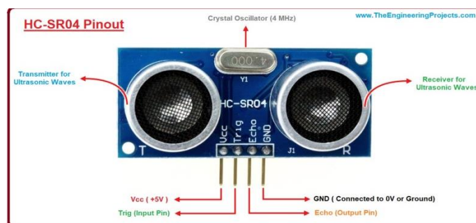
Figure.2 Block diagram of the Ultrasonic Sensor
