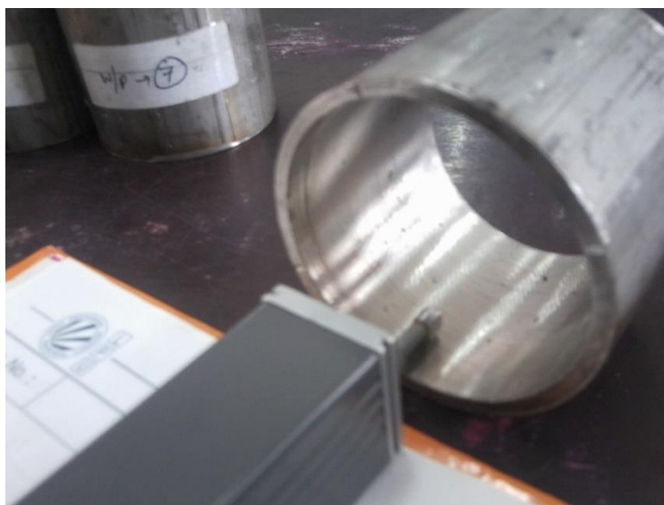
Fig 2: Surface roughness measurement using telesurf.
