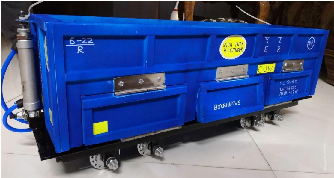
Fig.1. Prototype model of self-discharge railway wagon
