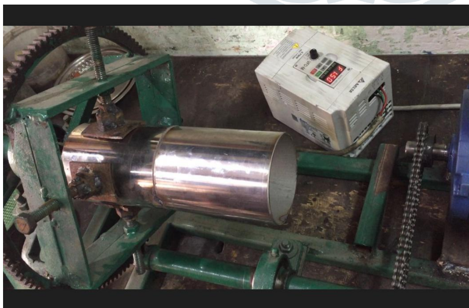
Fig 4. Fixture of automated TIG welding for circular section
