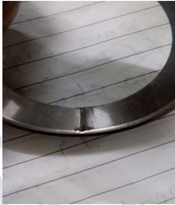
Figure 7: Outer race defect in taper roller bearing
