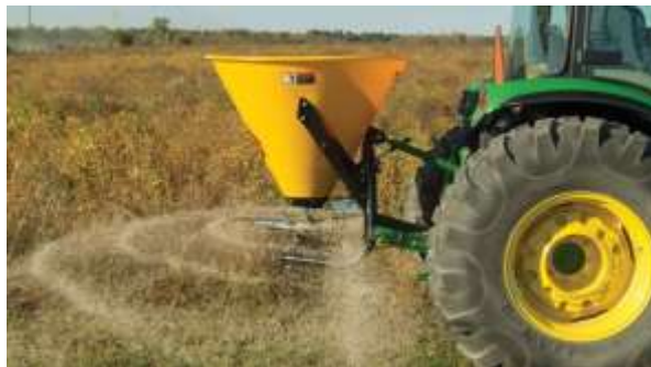
Figure 3: Impeller disc distributor
