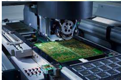
Figure 5: Automated machine used for manufacturing circuit boards from [4]
