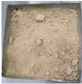
Figure 13: Pieces placed inside the sand for quenching at both temperature
