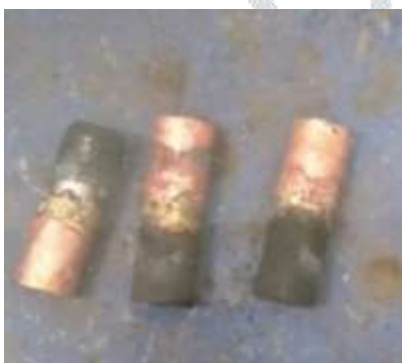
Figure 7: Water quenching ( 730^{\circ}\text{C} )
