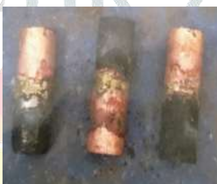
Figure 8: Water quenching ( 850^{\circ}\text{C} )
