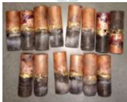
Figure 5: Welded Specimen with brass as filler material
