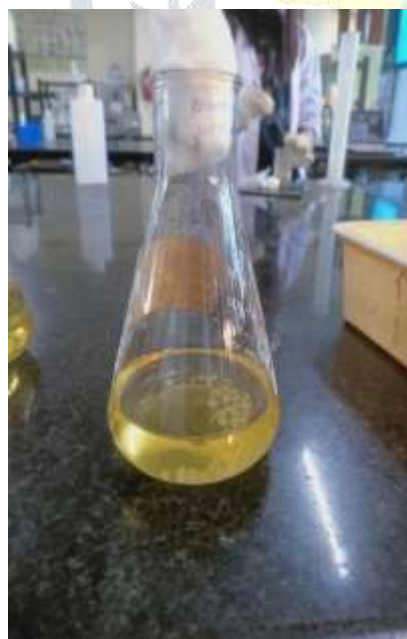
Fig. 29. Inoculation of formulated beads in the 100ml PD Broth in 250 ml of flask to check the stability of each hour used incubated shaker at 28°C.
