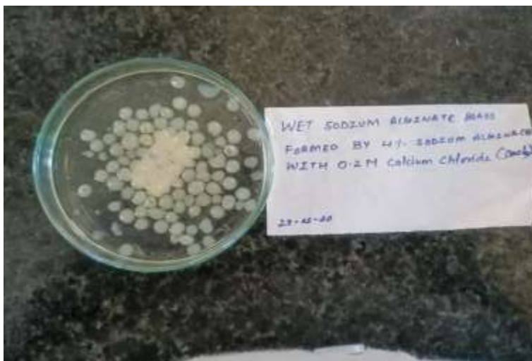
Fig. 28: Sodium Alginate Beads using 4% Sodium Alginate and 0.5 M Chloride.
