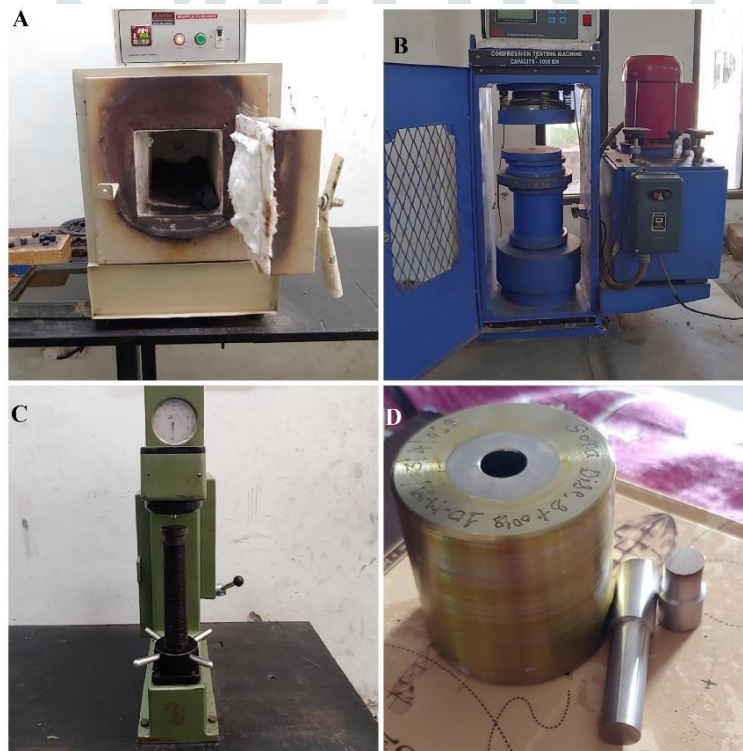
Figure 1 Muffle Furnace(A), Compression Machine-1000 kN (B), Rockwell Hardness Tester(C), Die and Punch(D)
