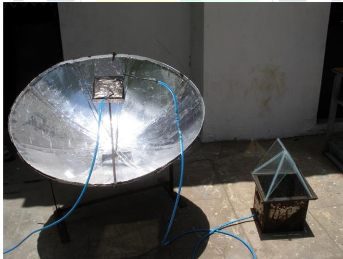
**Fig 2: Parabolic Dish Collector**
