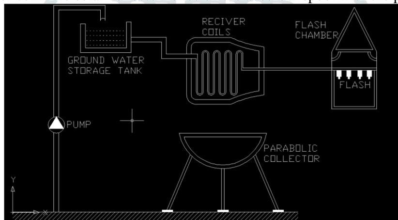
**Figure 1: Domestic Purpose Water treatment Plant**
