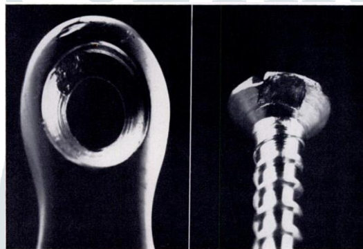
Figure 2. Head of screw and corresponding hole in plate to show face corrosion
