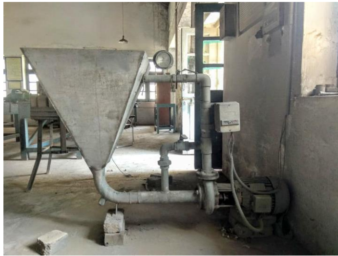
. Figure 3. shows the set up for slurry erosion testing.
