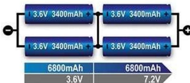
Fig 3: The above figure shows 4 cells arranged in series-parallel alignment.
