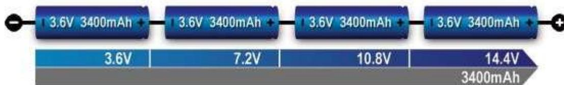
Fig 1: The above figure shows 4 cells connected in series.
