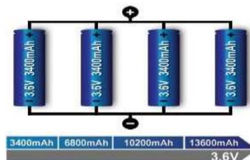
Fig 2: The above figure shows 4 cells connected in parallel.
