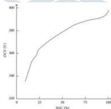
Fig 4: the above graph shows the non linear relationship between OCV and SOC for a lithium ion battery.
