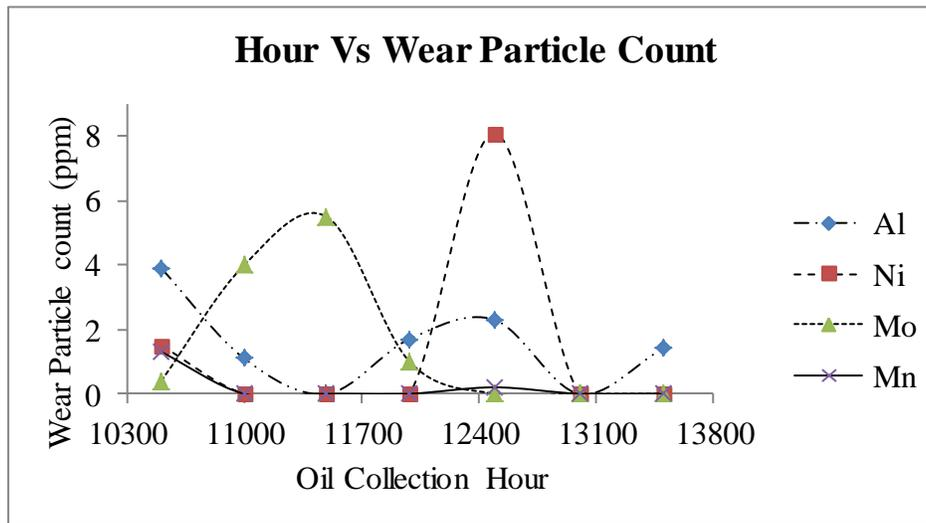
Figure 3: Wear Particle concentration of Al, Ni, Mo, Mn
