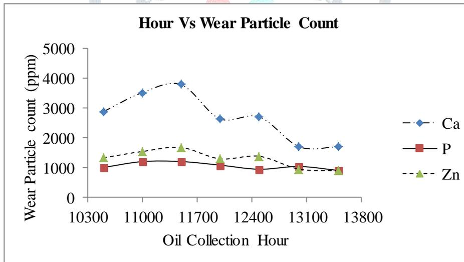
Figure 4: Wear Particle concentration of Ca, P, Zn
