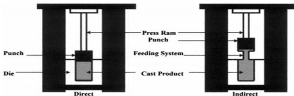
**Fig. 1 Schematic Diagram for Direct and Indirect Modes of the Squeeze Casting Process**
