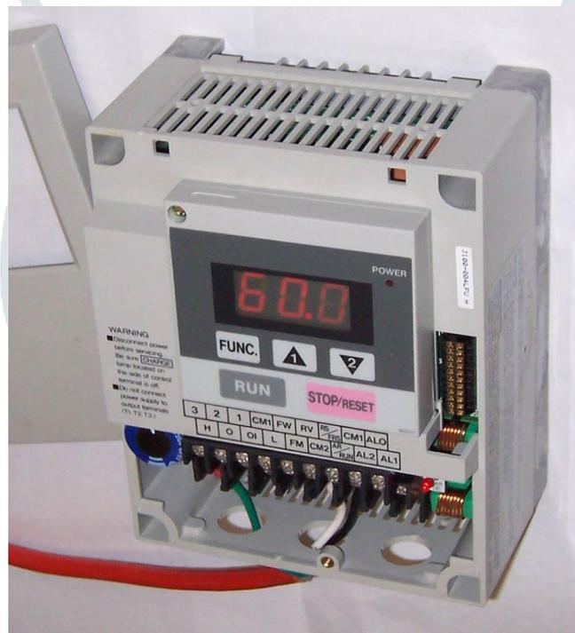
**Fig 1: Variable frequency Drive**
