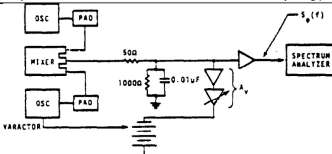
**Fig. 2:Second Differential Phase Commotion Estimation Set-Up**
