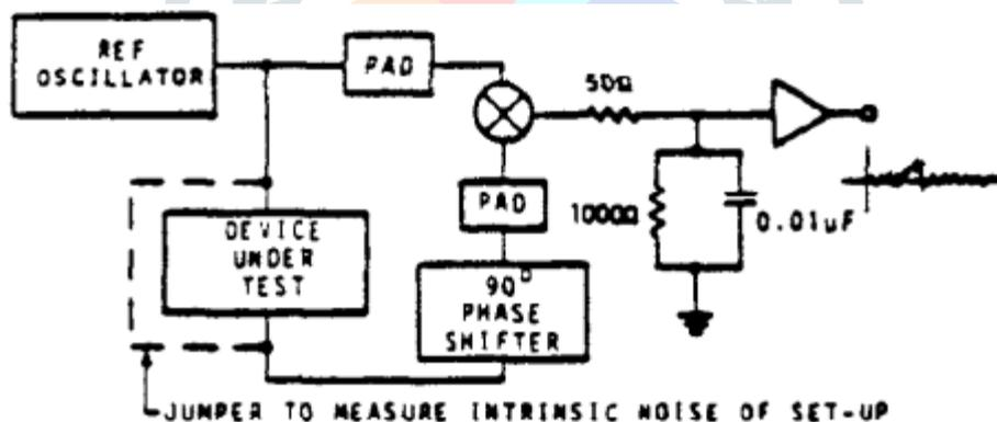
**Fig. 1: First Differential Phase Commotion estimation set-up**
