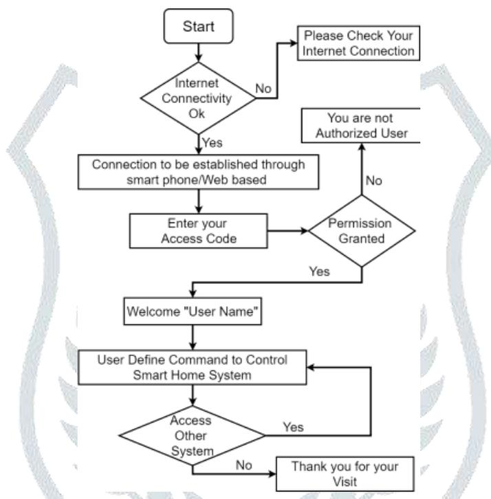
Figure 11 System flow on the smart home automation system using Google assistant
