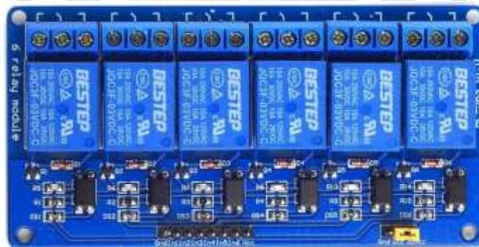
Figure 5. 6-channel 5 V DC relay module
