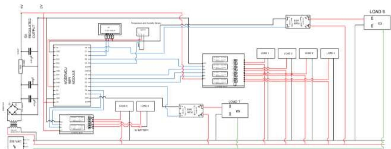
Figure 9. Circuit Diagram of the system
