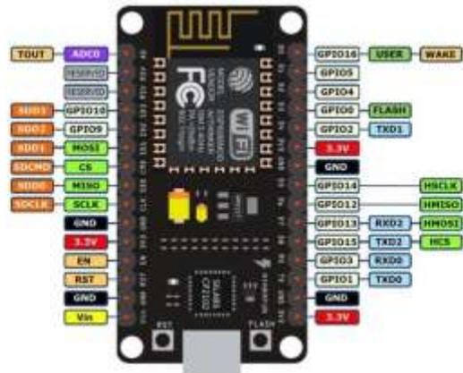
Figure 4 ESP 8266 Pin Diagram
