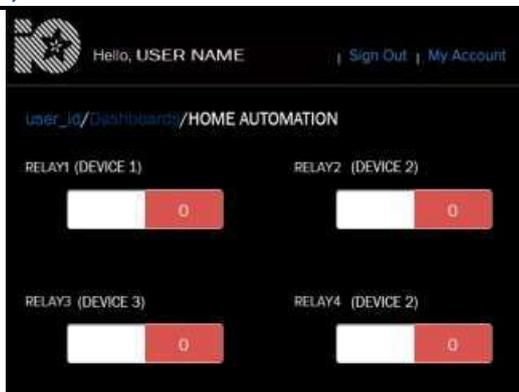
Figure 10 IoT home automation dashboard developed on Adafruit
