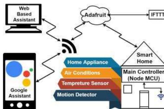
Figure 1 Smart home automation system architecture
