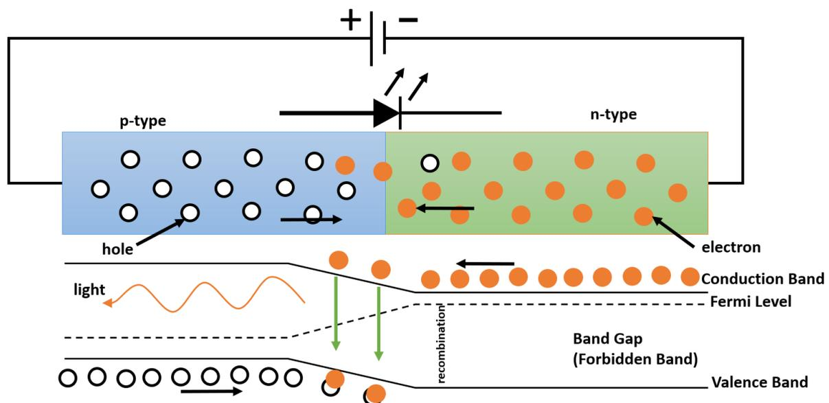
**Figure 4: Function and Energy Release in Light Emitting Diode by the Use of PN-Junction Diodes**
