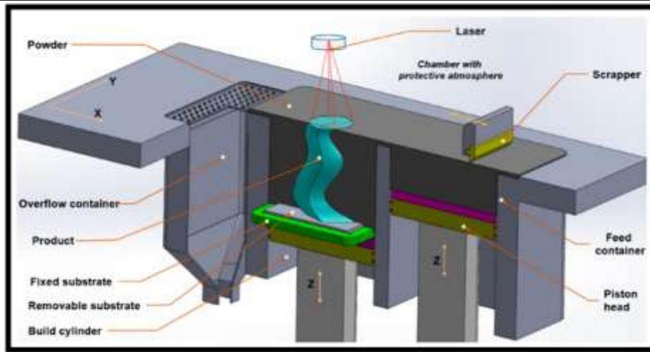
Fig. 2: Direct Metal Laser Sintering
