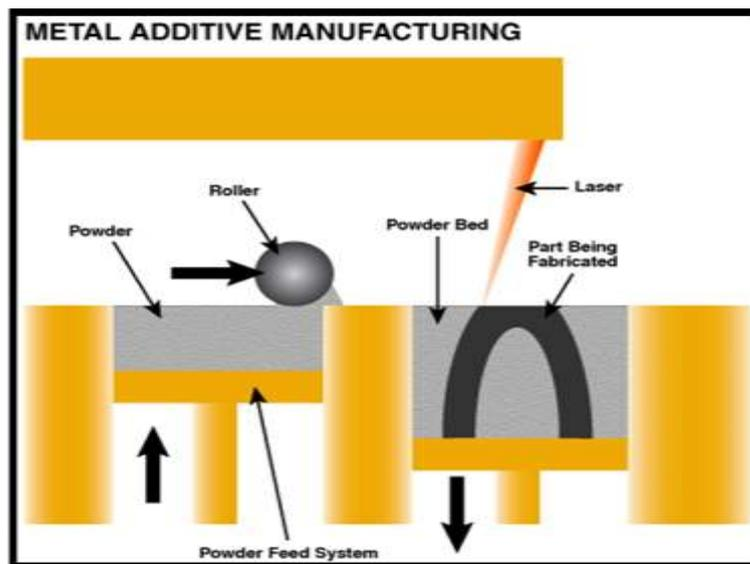
Fig. 3: Working of Direct Metal Laser Sintering
