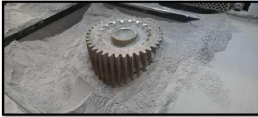
Fig. 1: Metal component produced by Additive Manufacturing.
