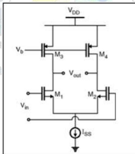
**Figure 2: Differential Amplifier with Current Source Load.**
