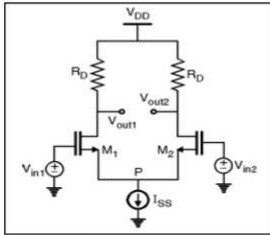
**Figure 3: The Basic Differential Amplifier.**
