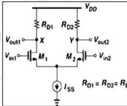
**Figure 4(a): Differential Amplifier with Passive Load and Current Source.**
