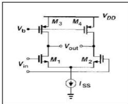
**Figure 4(b): Differential Amplifier with Active Load.**
