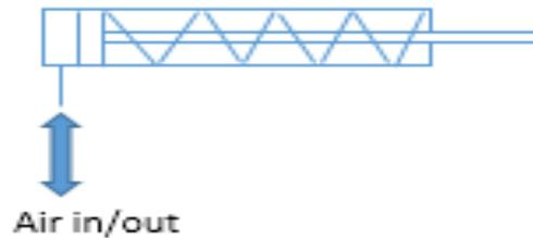
**Figure 3: Symbol used for single acting cylinder**
