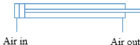
**Figure 4: Symbol used for double acting cylinder**
