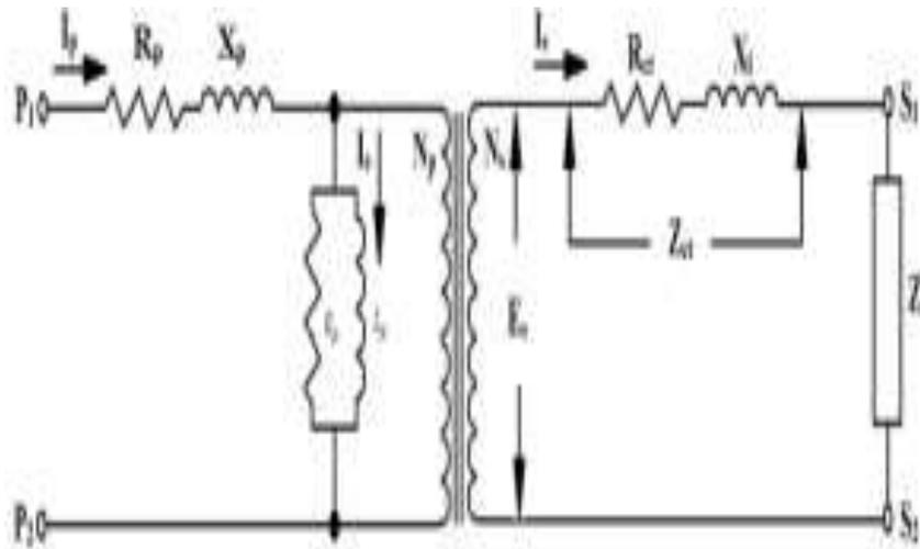
**Fig 1: Current Transformer Equivalent Circuit[3].**
