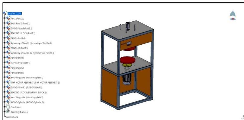
Fig. 2 Shows the actual design of m/c on Catia software
