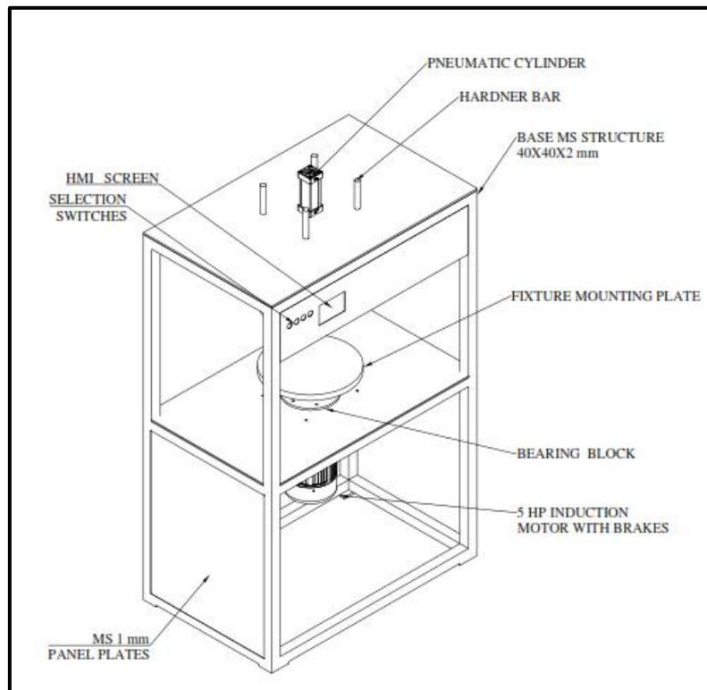
. Fig 3 shows the labelled diagram of machine
