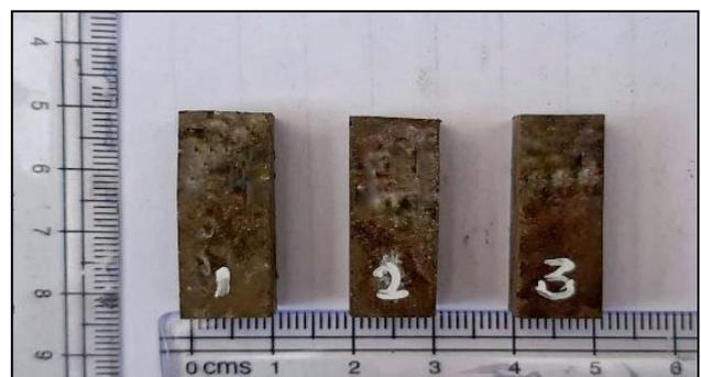
Fig. 6. Tribological testing specimens
