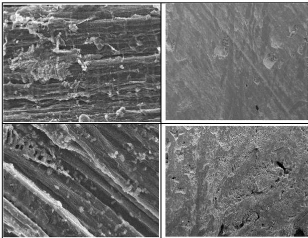
**Fig No. 10.** Surface Magnification Images of Hemp Fiber after NaOH treatment
