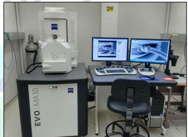
Fig. No. 9. Scanning Electron Microscopy (SEM)
