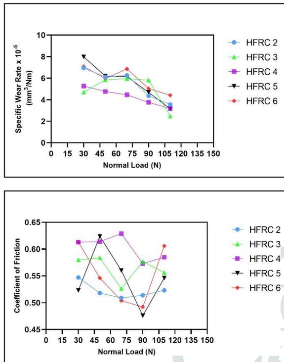
**Fig. No. 12.** SWR VS Normal Load and COF VS Normal Load (P-I)
