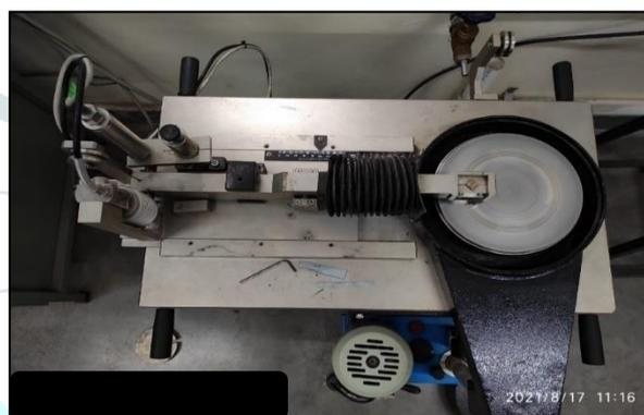
Fig. 7. Pin-on-disc setup
