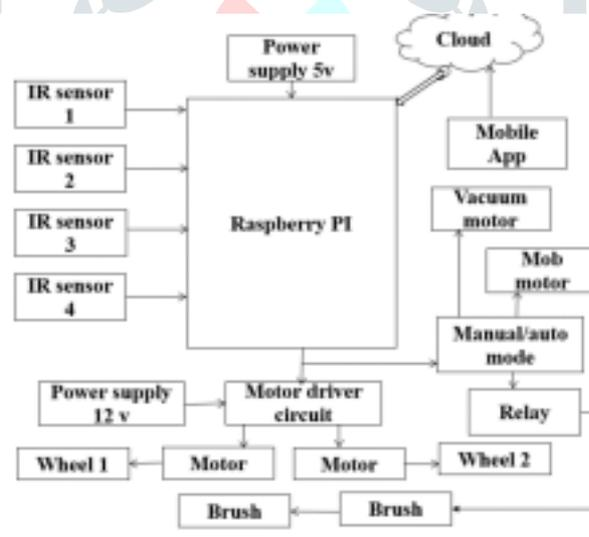
Fig. 1. Block diagram of automatic floor cleaning robot
