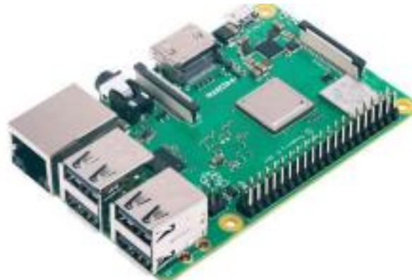
Fig 3.: Raspberry Pi 3B+ model
