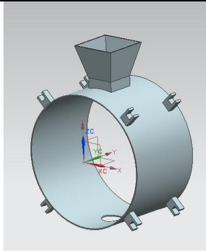
**Fig 3.** 3D Model of heating and mixing chamber
