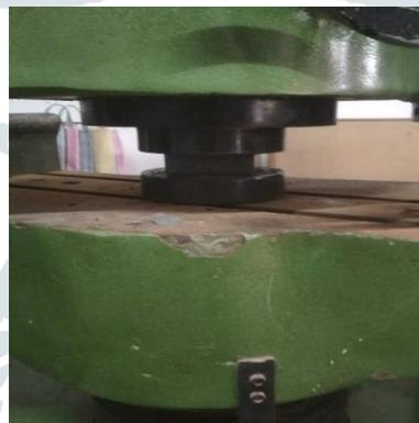
Fig 2. Testing of block under Compression Test
